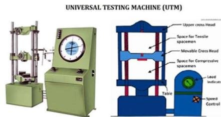
Fig.4.3. Universal Testing Machine
