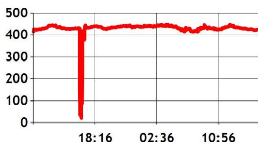
RMS VOLTAGE VARIATION TIME PLOT OF CH3
