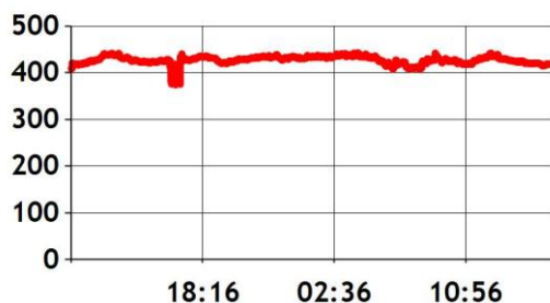
RMS VOLTAGE VARIATION TIME PLOT OF CH2
