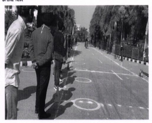
Our bike was practically tested on Day 3. First of all it was the brake test for which we had to fully accelerate our bike for about 300 m and then suddenly apply the brake to stop before the dotted line.
