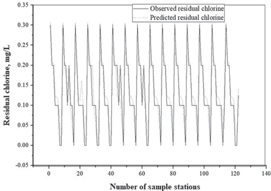
Figure 12. Prediction of residual chlorine at sample station by FFNN (2-25-1) LM model.
