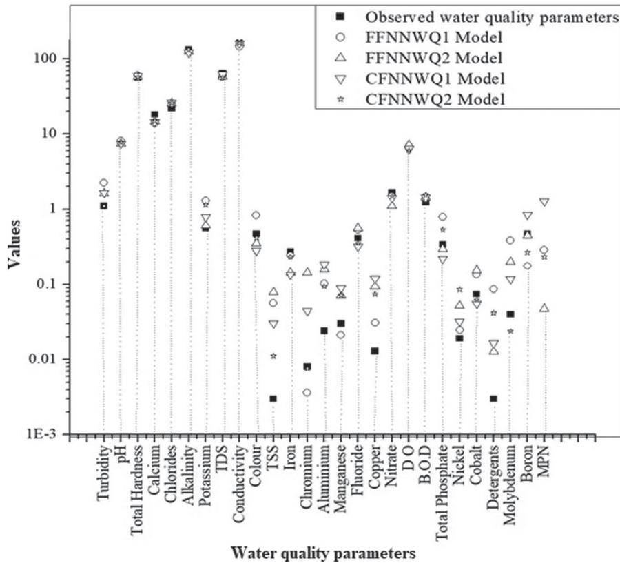
Figure 8. Prediction of water quality parameters by various types of ANN models.
