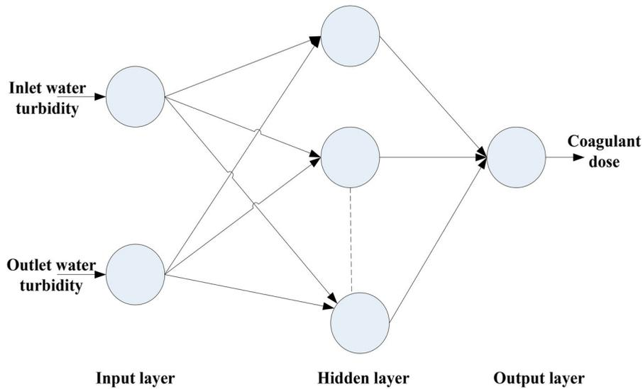
Figure 3. Coagulant dose neural network model.
