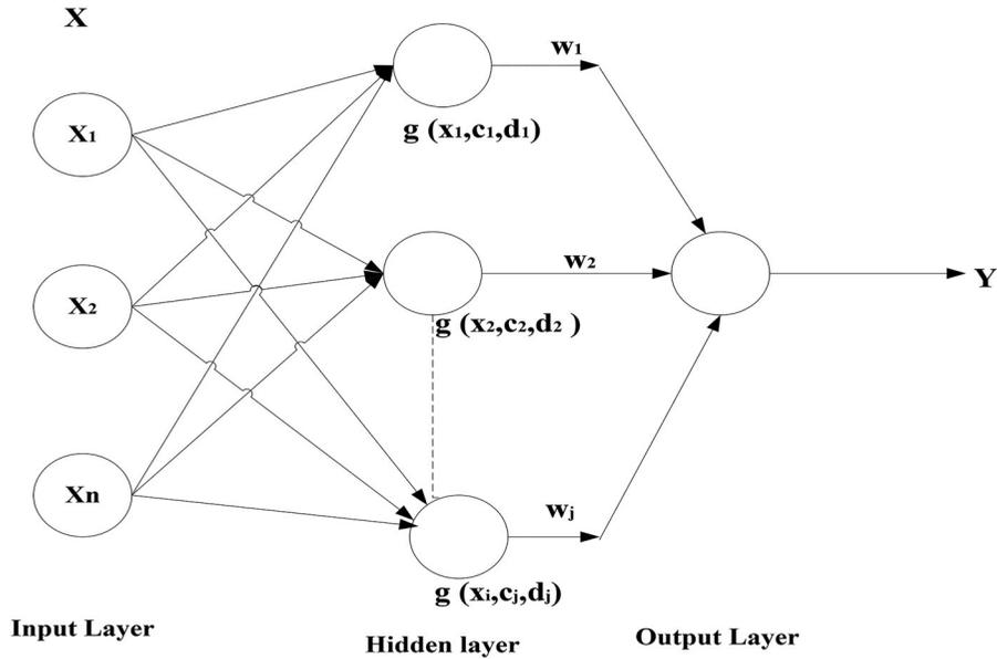
Figure 1. A typical radial basis function neural network.
