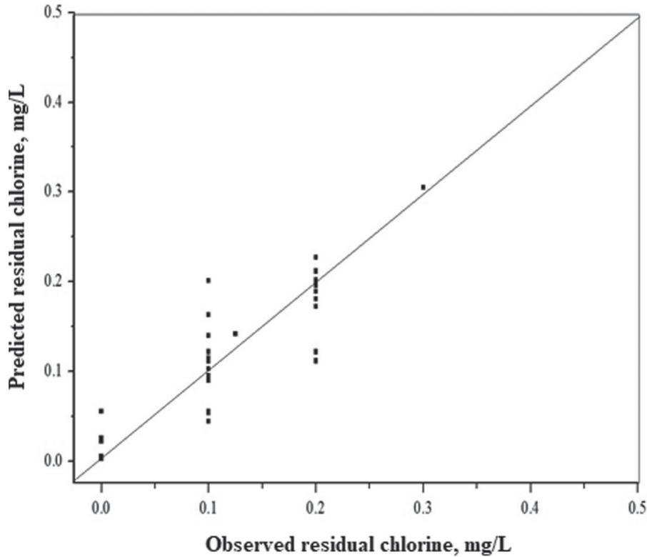
Figure 13. Scatter plot of FFNN (2-25-1) LM model during training and testing period.
