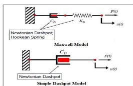
In this model, the spring attached in parallel to the dash-spot
