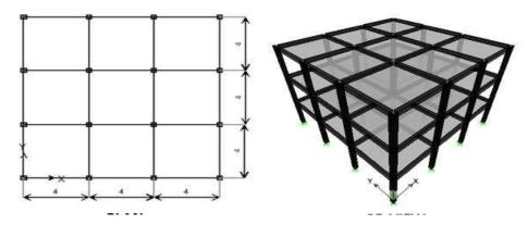
Manual calculate axial load =747 KN (factored)
