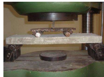
Fig 3.4.2 Testing of panel
