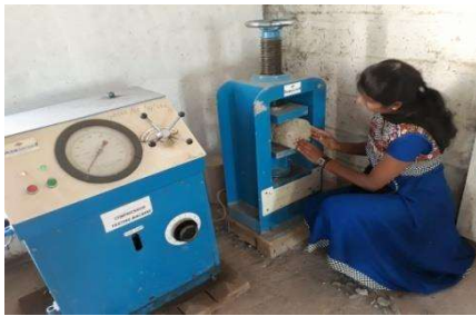
Fig.3 Split tensile strength Test specimen
