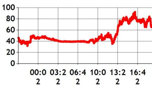
TOTAL APPARENT POWER VARIATION TIME PLOT
